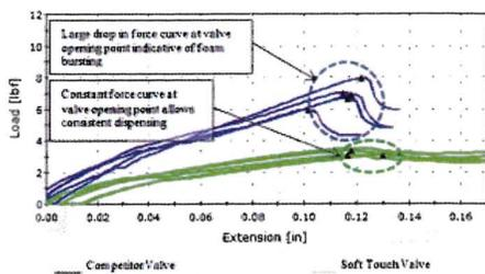
Figure 1 - Force Curve for OCF Valve Opening
