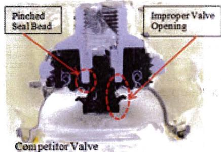
Figure 3 - Competitor's Valve Damaged from Improperly Dimensioned Dispensing Gun Basket
