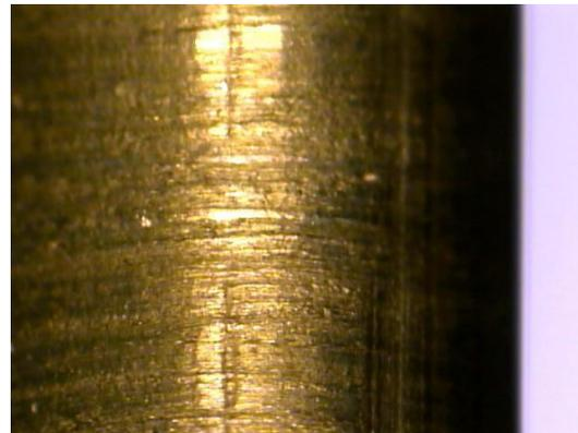
Figure 5: Bead of an Aluminum can magnified 88X showing eyelashing
