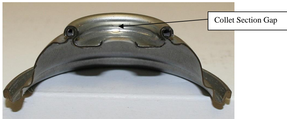
Figure 13 – Gap on Crimp between Collet Sections
