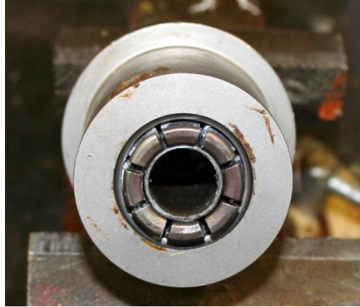
Figure 22 – Expanded Collet showing Gap between Sections
