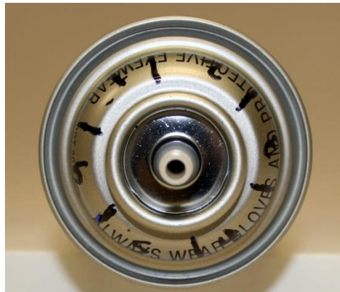
Figure 23 – Top of dome after Marking and Numbering Collet Sections
